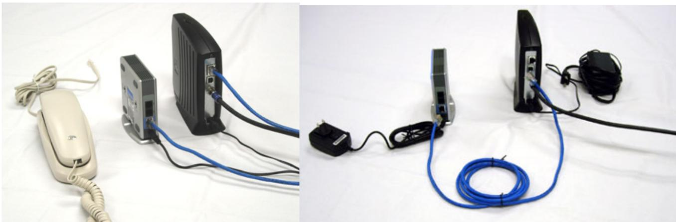
**Step 3:** This step shows a phone plugged into port 1 on the back of the Pap2, by default this the port into which you will plug your telephone. At this point you should have 3 lights lit on the Pap2 device, the top light for power, second is the Ethernet connectivity, and the bottom light should also be lit indicating that the phone is plugged in. You should be able to make calls at this point.
