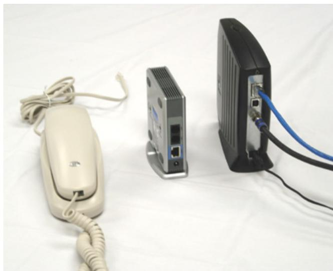
**Step 2:** The picture below shows the connection directly from your modem (DSL or Cable apply). In this step you will take the cable that is currently going to the computer from the modem and plug into our device the pap2. The picture shows the blue cable coming from the modem and plugging into the blue port on the back of the Pap2, marked Ethernet. The picture to the Right is showing the connection without either device plugged into the wall outlet for power. This is just an example.
